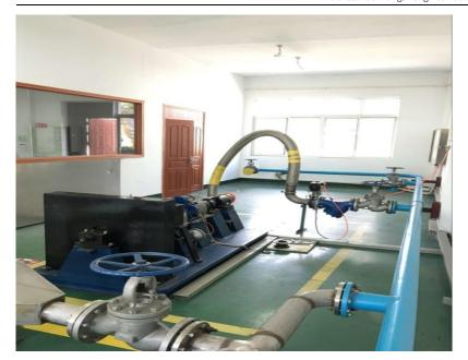
The test bench can perform full function test on ATS of civil and military aircraft currently in operation in China, including B737, B747, B777, A320, A330, MA700, etc. The flywheel loading mode is adopted, or other loading modes can be selected according to the user's budget and technical requirements.
